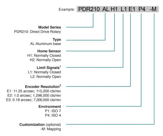
Notes: 1) The PDR series does not include limit sensors. The Limit Signal options are provided for compatibility with motion controller requirements. 2) Standard encoder max output frequency is 12.5 MHz.
