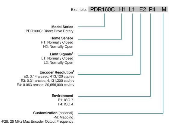
Notes: 1) The PDR series does not include limit sensors. The Limit Signal options are provided for compatibility with motion controller requirements. 2) Standard encoder max output frequency is 12.5 MHz.
