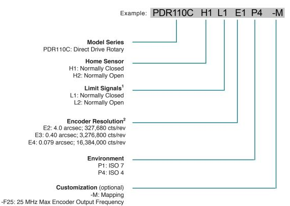
Notes: 1) The PDR series does not include limit sensors. The Limit Signal options are provided for compatibility with motion controller requirements. 2) Standard encoder max output frequency is 12.5 MHz.
