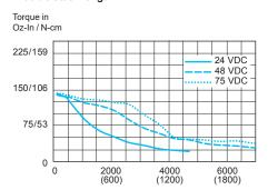
Speed of rotation in full steps per second (rpm)
