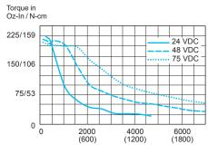
Speed of rotation in full steps per second (rpm)
