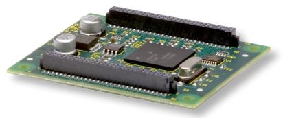
A PC board-mounting card for adding I/O to a CAN distributed control network. The CAN-IPM-01 combines configurable digital I/O points with dedicated analog and digital inputs and outputs to enhance distributed control networks using Copley's CANopen servo drives and stepper drivers.
