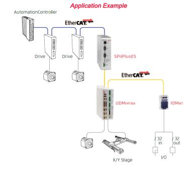
The SPiiPlusES is a high performance programmable motion controller and EtherCAT Master that can be connected as a node to any EtherCAT network utilizing the standard DS402 CAN Over EtherCAT (CoE) protocol. To the external EtherCAT Master it looks like a highly programmable multi-Axis motor drive.
